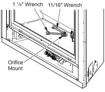
Figure 55 - Removing Main Burner Orifice
